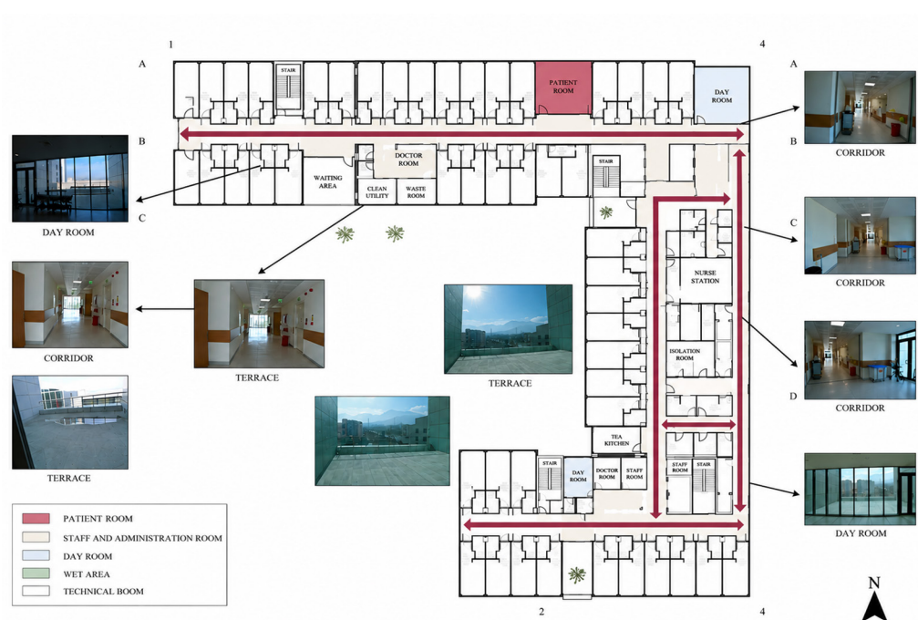
Figure 5. Floor Analysis of Balcony-2 (reproduced by authors).
