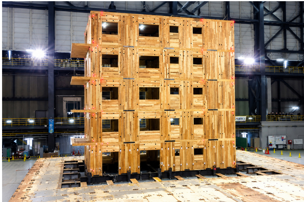
Figure 1. Earthquake shake table tests of a cross-laminated timber (CLT) earthquake-resistant building (UL Solutions, 2023).
